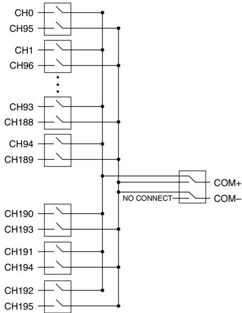
Figure 2 shows the NI 2575 connector pinout for the 1-wire 196 × 1 topology.
