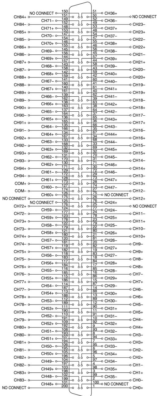
Figure 4 shows the NI 2575 connector pinout for the 2-wire 98 × 1 topology.
