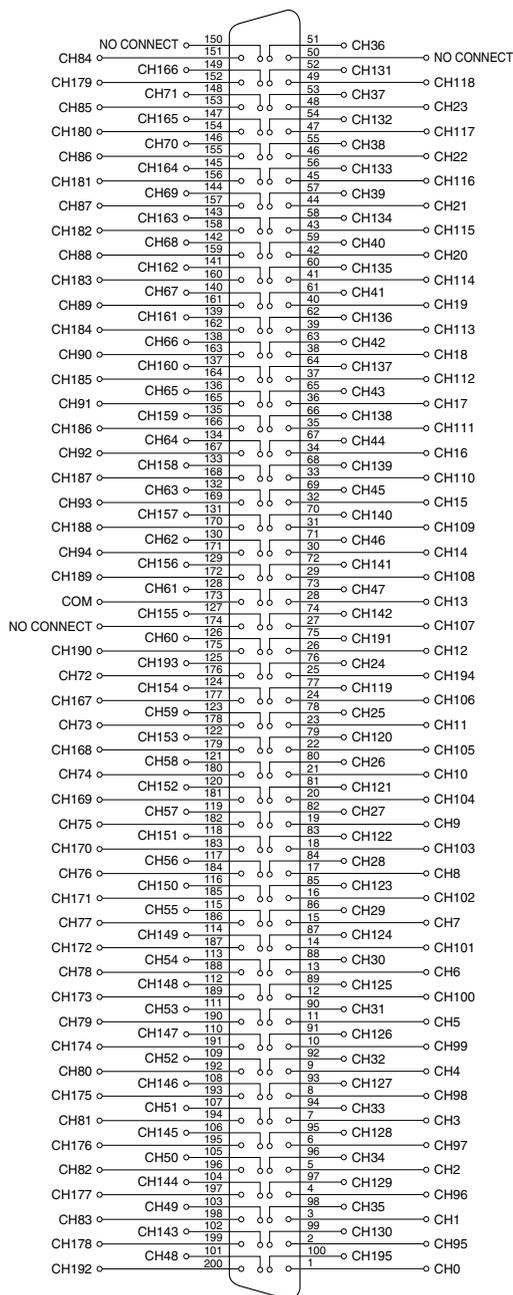
Figure 3 shows the NI 2575 connector pinout for the 2-wire 95 × 1 topology.
